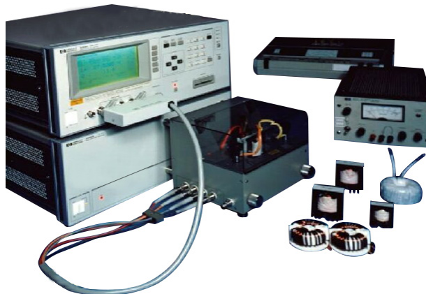
Measurement using 42841A bias current source
